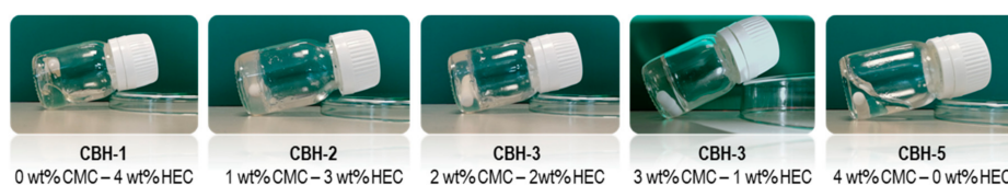
Figure 2. Digital images of gel appearance as a function of the cellulose derivatives' weight ratio. CBH is the abbreviation for cellulose-based hydrogel; CMC for carboxymethyl cellulose and HEC for hydroxyethyl cellulose.
