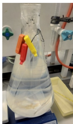
Figure 2. Dialysis of GelMA against DI at 50 °C for 1 week; three dialysis bags are shown in this figure.
