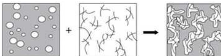
Effect of the CNT dispersion (at low contents) on the morphology of the PPS/PA66 60/40 blend. Image obtained from reference 210.
