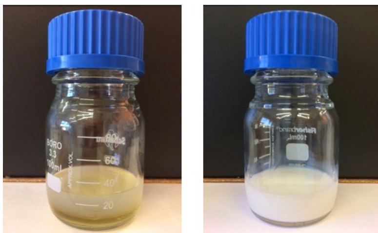
Figure 34. Photographs of the dispersion obtained from WNIPU3 after acetone removal (left) and WNIPU4 one year after acetone removal (right).
