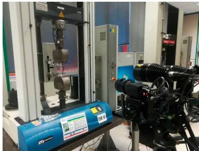
Figure 9. Digital image correlation (DIC) optical system.
