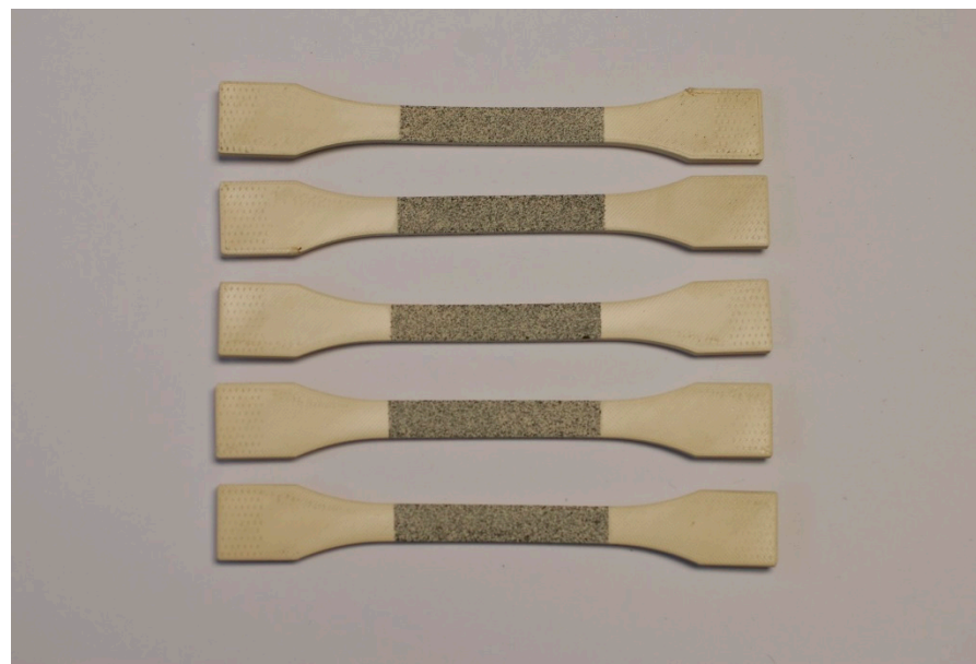
Figure 7. Printed samples for tensile test.
