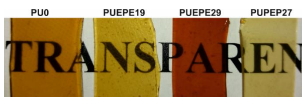
Figure 4.3. Visual appearance of triblock copolymers based waterborne poly(urethane-urea) films. PU0 film was added for comparison purpose.
