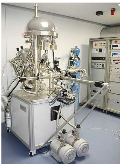
Figure A.2.7. SPECS system equipped with Phoibos 150 1D-DLD analyser.
