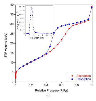
**Figure 4.** N<sub>2</sub> isotherms and pore size distribution (inset). The pore size distribution was modelled using DFT fitting: (**a**) PPC-0; (**b**) PPC-ALS; (**c**) PPC-CTAB; (**d**) PPC-TWEEN.
