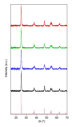
**Figure 1.** PXRD patterns of PPCs (pink line: Simulated PXRD from the crystallographic information file retrieved in the Inorganic Crystal Structure Database for anatase ICSD no.: 024276; black line: PPC-0; blue line: PPC-ALS; green line: PPC-CTAB; red line: PPC-TWEEN).
