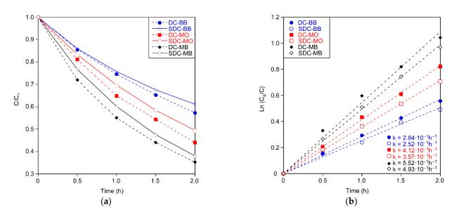
**Figure 10.** (a) Comparison of evolution of the relative dye concentration between different applications methods. (b) Fitting of the dye photodegradation to the first-order kinetic model, showing the resulting rate constants. Blue circles: remazol black B (BB); red squares: methyl orange (MO); black rhombuses: methylene blue (MB). Filled figures: dip coating (DC); empty figures: slot-die coating (SDC).
