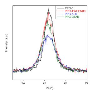
Figure 2. Excerpt of the PXRD patterns showing the broadening of (101) reflection.
