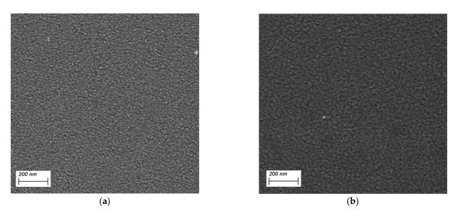
Figure 6. SEM image of surface morphologies: (a) PPC-ALS and (b) PPC-0.
