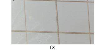
**Figure 11.** (a) Surface profile of DC (dip coating) and SDC (slot-die coating) coatings obtained by profilometry. (b) Microscope image of the sample SDC after the cross-cut test.
