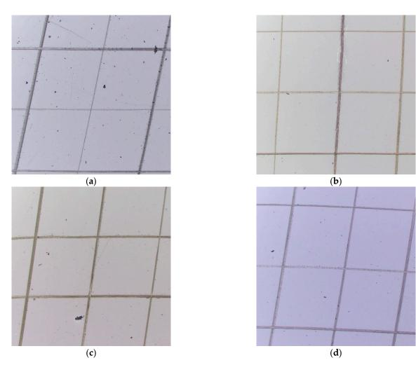
Figure 7. Microscope images of the samples after the cross-cut test: (a) PPC-0; (b) PPC-ALS; (c) PPC-CTAB; (d) PPC-TWEEN.
