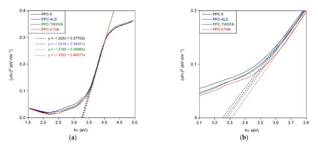
**Figure 5.** (a) Tauc plots of TiO<sub>2</sub> layers. The linear part of the plot is extrapolated to the abscissa axis. (b) Enlarged section of the linear part extrapolated to the x-axis.
