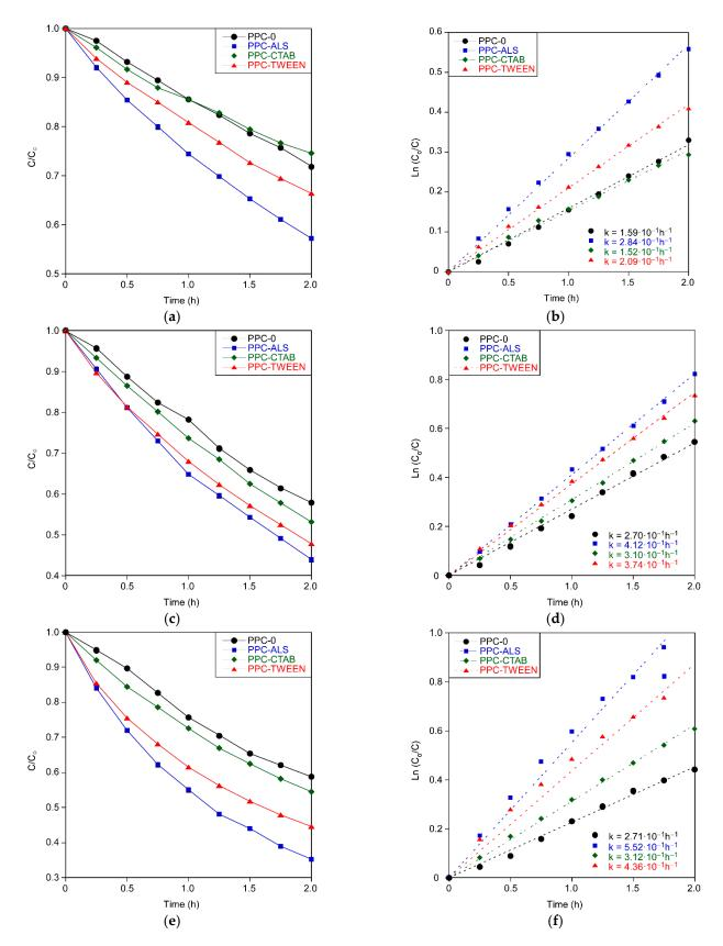
**Figure 8.** Evolution of the relative dye concentration for the photocatalytic coatings with diferent surfactants. Fitting of the dyes' photodegradation to the first-order kinetic model, showing the resulting rate constants for all coatings: BB photocatalysis (**a**) and kinetics (**b**); MO photocatalysis (**c**) and kinetics (**d**); MB photocatalysis (**e**) and kinetics (**f**).
