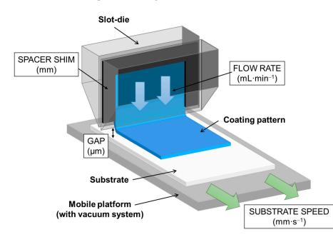
Figure 12. Diagram of the slot-die process and coating parameters.
