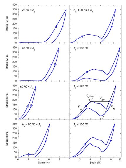
**Figure 1.** Stress–strain compression curves at different temperatures: below  $A_s = 69 \,^{\circ}$ C, in the interval  $A_f$ - $A_s$ , where  $A_f = 92 \,^{\circ}$ C, and above  $A_f$  of the thermally induced reverse MT. The schematic at temperature 120  $^{\circ}$ C shows how the values of critical stress ( $\sigma_{critical}$ ), superelastic strain ( $\varepsilon_{SE}$ ), and Young's moduli of the austenitic ( $E_A$ ) and martensitic ( $E_M$ ) phases were determined.
