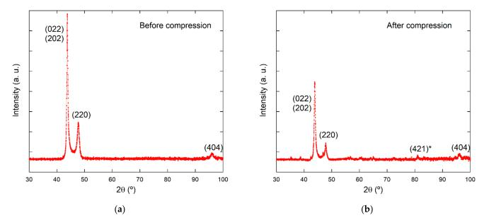
**Figure 4.** X-ray diffraction patterns of the basement surface of the sample in the martensitic state measured at room temperature: (**a**) before thermomechanical testing and (**b**) after the thermomechanical treatment.
