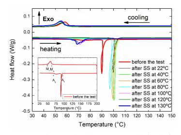
**Figure 3.** DSC heating and cooling runs measured before the first stress–strain (SS) test and after each compression SS cycle at the constant temperature indicated in the graphs. The inset illustrates the determination of the MT characteristic temperatures in the as-received sample before testing for which the two-step reverse MT is observed on the heating curve (see experimental section).
