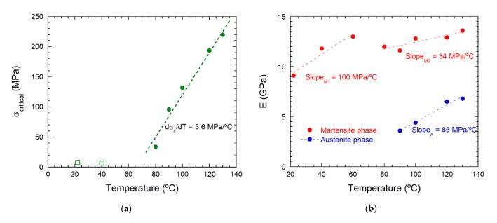
**Figure 2.** (a) Temperature dependence of the critical stress of the MT start (solid circles) and twinning stress (open squares). (b) Evolutions of Young's moduli,  $E_A$  and  $E_M$ , with the temperature. All lines are the linear fits to the data points.
