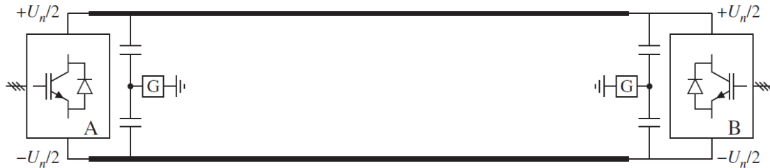
Figure 12 Symmetrical monopolar configuration
