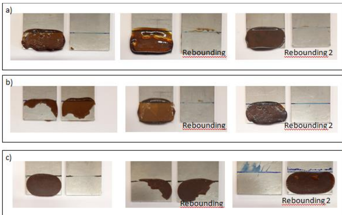
Figure 18. Photos of the representative adhesion failure of the adhesives applied at 80°C for a) 70/30-MXDA; b) 60/40-MXDA and c) 50/50-MXDA.
