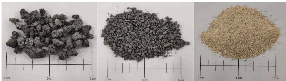
Fig. 1. Used aggregates: EAFS 4/12 mm (left); EAFS 0/4 mm (middle); limestone fines 0/1.18 mm (right).
