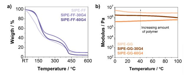
**Figure 2.** a) Thermal gravimetrical analysis (TGA) curve of SIPE-FF-x family of electrolytes undertaken under nitrogen atmosphere and 10  $^{\circ}C \cdot min^{-1}$ ; and b) Dynamic mechanical thermal analysis (DMTA) of SIPE-GG-x family membranes at compression from 0 to 100  $^{\circ}C$ .
