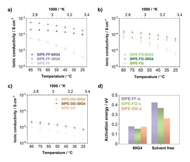
**Figure 3.** Ionic conductivity values at different temperatures of a) SIPE-FF-x electrolytes containing increasing amounts of tetraglyme (G4) plasticizer, b) SIPE-FG-x electrolytes family and c) SIPE-GG electrolytes family; d) Activation energies (eV) calculated following Arrhenius fittings of thermally-activated processes[30].
