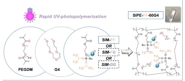
**Scheme 2.** Lithium single-ion polymer electrolyte (SIGPE) synthesis process by UV-photopolymerization. SIPE-FF-60G4 chemical structure is illustrated as an example.
