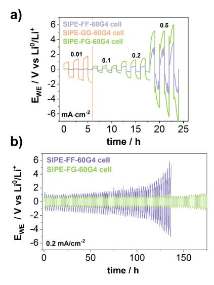
**Figure 6.** a) Lithium stripping/platting curves at increasing current densities from 0.01 to 0.5 mA·cm<sup>-2</sup> in symmetrical lithium cells of SIPE-FF-60G4 cell, SIPE-FG-60G4 cell and SIPE-GG-60G4 cell; and b) Long cycling of Li/Li cells at 0.2 mA·cm<sup>-2</sup>.
