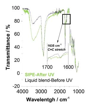
**Figure 1.** FT-IR spectra of a SIGPE membrane before (black line) and after (green line) UV-photopolymerization. *Inlet*: disappearance of the band associated with the carbon double bond of acrylic functionalities (1635 cm<sup>-1</sup> band)[26] after UV irradiation.
