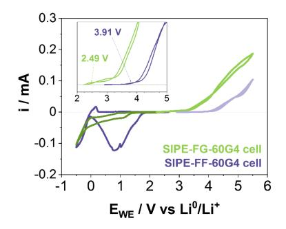
**Figure 5.** Voltammograms of SIPE-FG-60G4 and SIPE-FF-60G4 electrolytes at 60  $^{\circ}$ C and a scan rate of 0.2 mV·s<sup>-1</sup>. Scans were undertaken in Li<sup>0</sup>/Cu<sup>0</sup> (from OCV to -0.5 V) and Li<sup>0</sup>/Stainless steel (from OCV to 5.5 V) cells.
