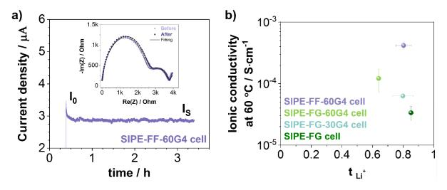
**Figure 4.** a) Chronoamperometry plot for the lithium transference number calculation following the Evans-Vincent-Bruce method[31] of SIPE-FF-60G4 electrolyte. *Inlet*: Nyquist impedance plots before and after polarization, including fitting curves by equivalent circuits; and b) Ionic conductivities against lithium transference number of SIPE-FF-60G4 electrolyte and SIPE-FG-x family of electrolytes containing different amounts of G4 plasticizer.
