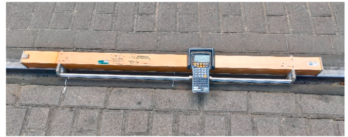
Fig. 4. Corrugation measurement device (R2S).
