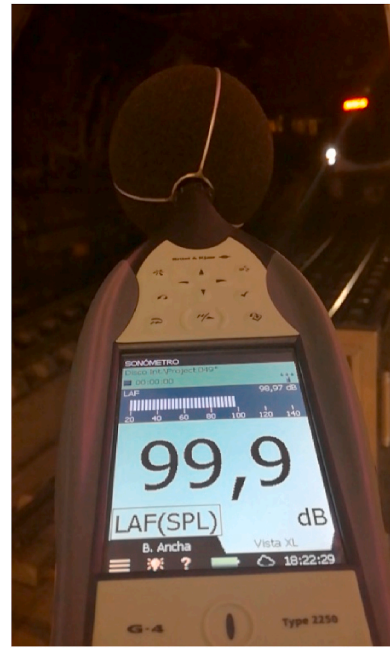
Fig. 1. Measured noise level in a station.
