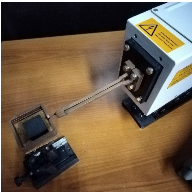
Fig. 10 Picture of the dedicated inductor with one of the samples in place
