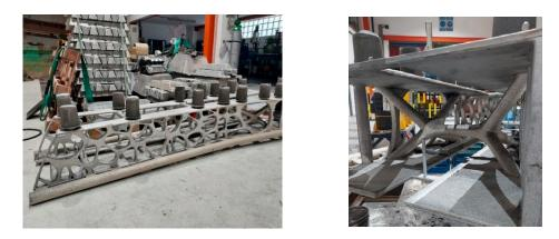
**Figure 17.** Part manufactured after the demolding. Filling and feeding systems are also shown in this image at Tecnalia's facilities (**left**). Inner Skeleton features (**right**).
