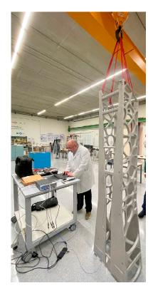
**Figure 18.** Modal test configuration for free vibration conditions with the data-acquisition device, the accelerometer in the top right area of the part, and the hammer at UPV/EHU's facilities.
