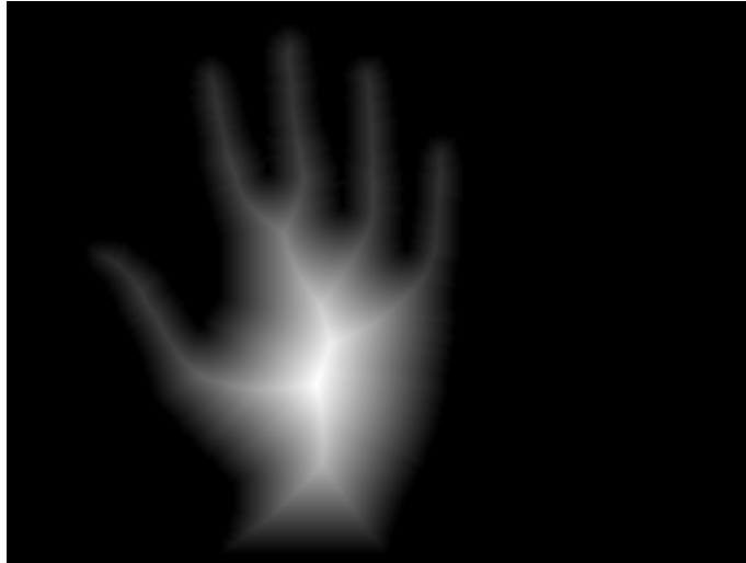
Figure 3.9: Visual representation of the Distance Transform of an open hand shape. The gray level indicates the DT value. Brighter corresponding to higher DT value. A contrast enhancement has been performed on this image.
