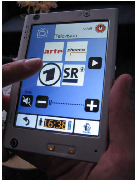
Figure 3.6: Multimodal UI based on gesture and speech interaction running on a PDA controller: HTC 7500 Advantage. The GUI implements the requirements posed by a young person with cognitive impairments.
