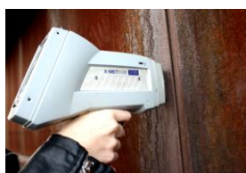
Figure 1. XRF in situ analyses on the water runoff and summary of the XRF results (% w/w) of the reddish and grey areas formed as a consequence of water runoff.
