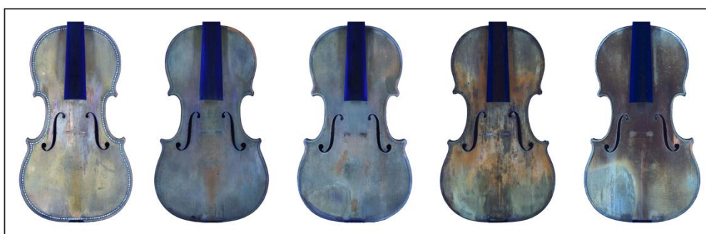
Figure 1. UVIFL photos of Antonio Stradivari ("Hellier" 1679, "Ford" 1703, "Cremonese" 1715), Guarneri "del Gesù" ("Principe Doria" 1734) and Jean-Baptiste Vuillame (copy of Messiah 1870) violins
