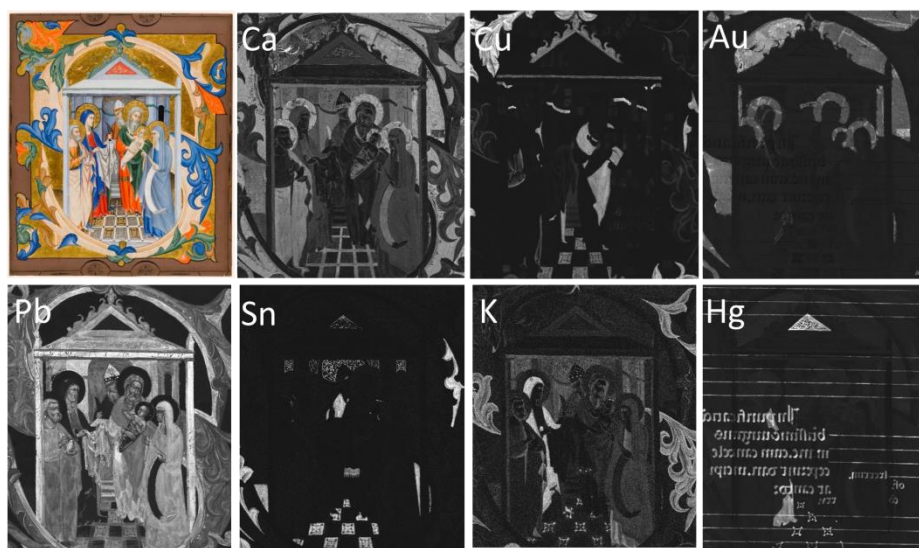
Figure 1. MA-XRF images of one of the investigated samples at the Fitzwilliam Museum.
