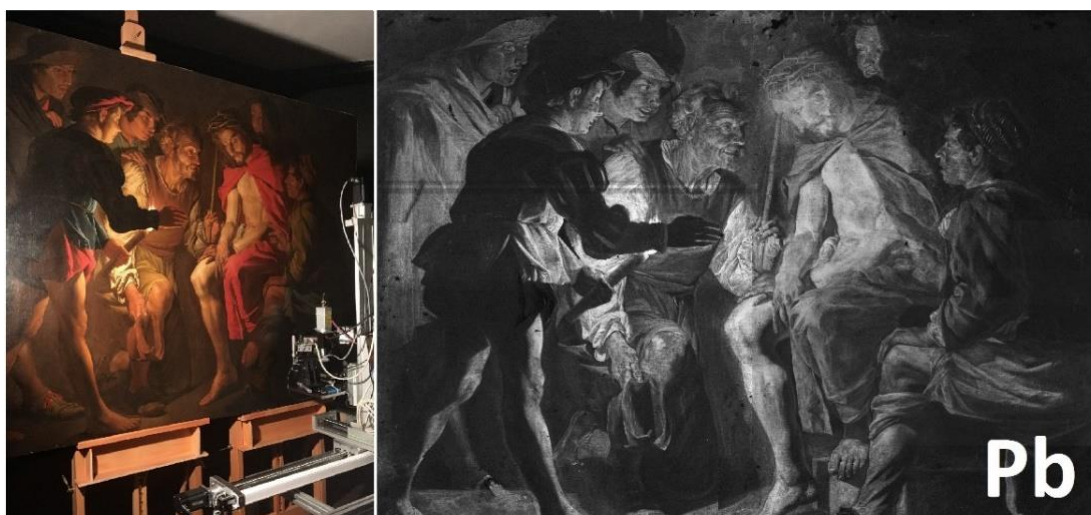
Figure 1. The Mocking of Christ (1640, oil on canvas 200x155 cm) by Matthias Stomer during the MA-XRF scanning; the scanning of the full painting lasted 8 h (left). The elemental distribution image of Pb evidencing a "pentimento" in the pictorial composition of the face of Christ (right).
