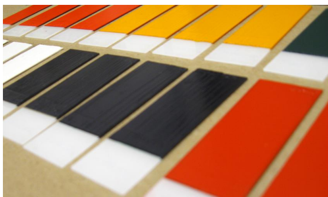
Figure 1. Some of the paint-outs of water-mixable oil paints used in this study.
