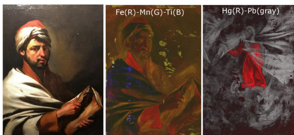
Figure 1. “The prophet” by Jusepe de Ribera (ca. 1620). MAXRF scanning allowed identifying original pigments, restorations with modern pigments and the presence of a hidden painting below the visible surface depicting a woman in adoration.
