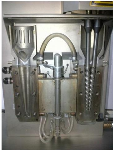
**Figura 3.1.** *Twin screw compounder DSM Xplore.*
