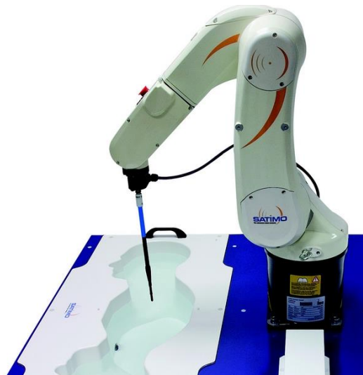
Figure 2.6. System for assessing SAR.
