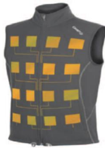
Figure 5.13. Vest with receiver antenna array proposed in (Vitas 2014).
