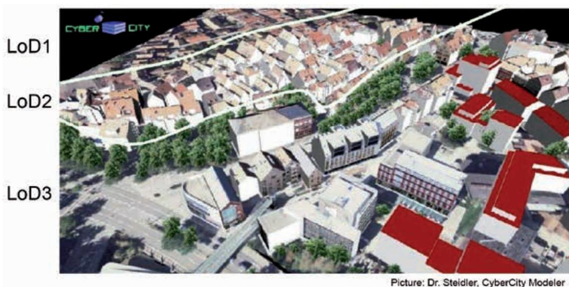
Figure 11: Different Levels of Detail in a scene.
