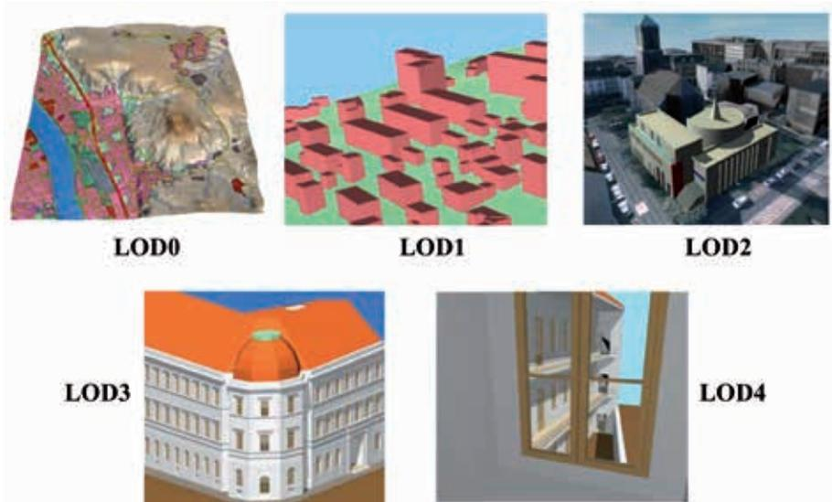
Figure 10: The five levels of detail (LoD) defined by CityGML.
