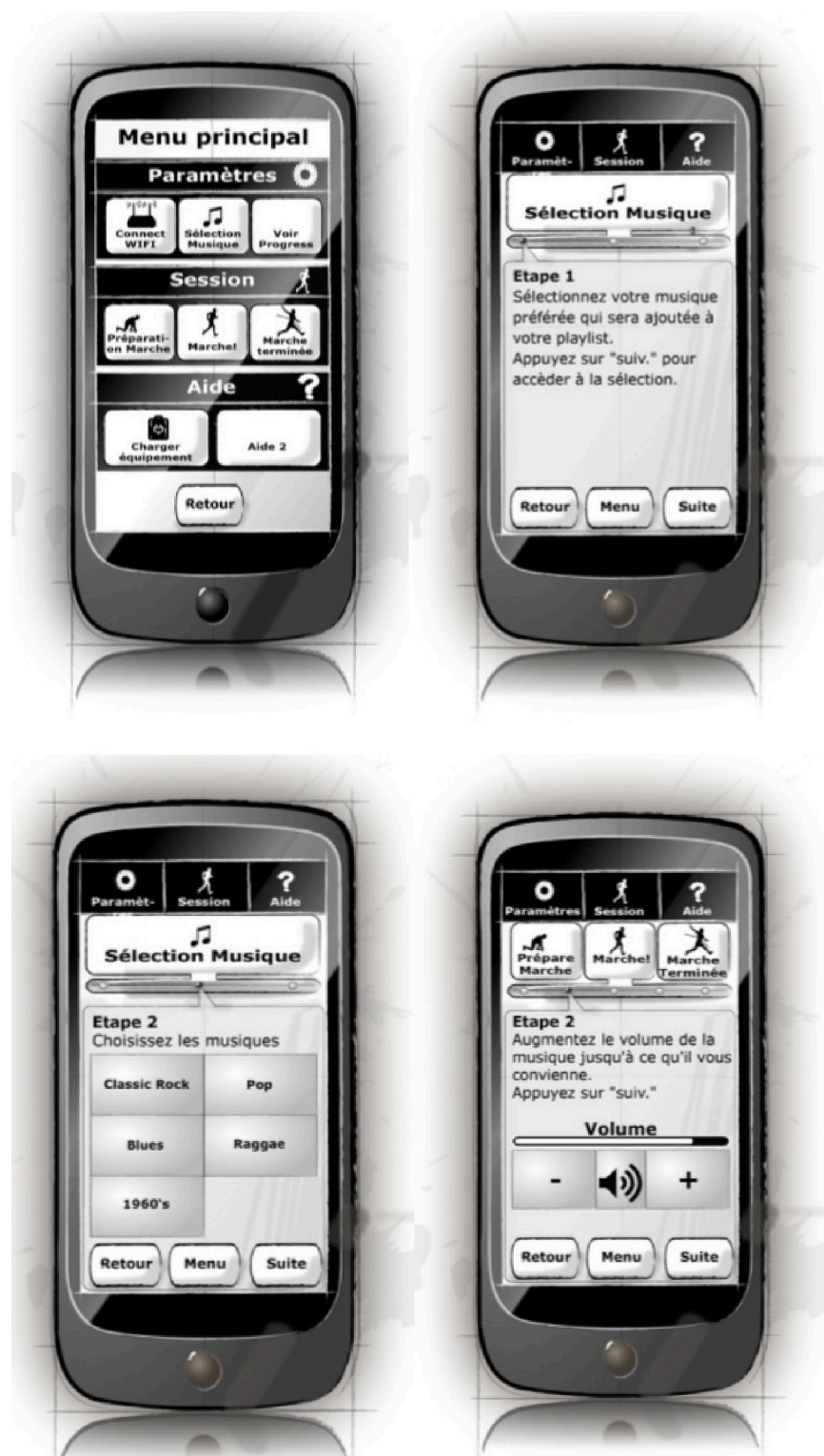
Fig 7. Paper prototype screens used in the Wizard-of-Oz mobile application mock-up evaluated in the first iteration.
