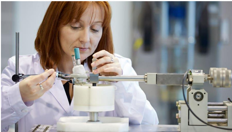
Figure 2. 4 MicroTest MT/10/SCM tribometer with the electrodes installed for the tribocorrosion test.
