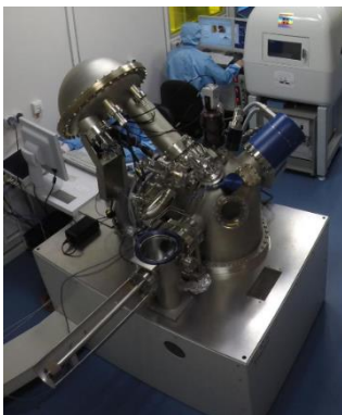
Figure 2. 10 - XPS Thermo Fisher Scientific Theta Probe (East Grinstead, United Kingdom) at AC2T research GmbH.
