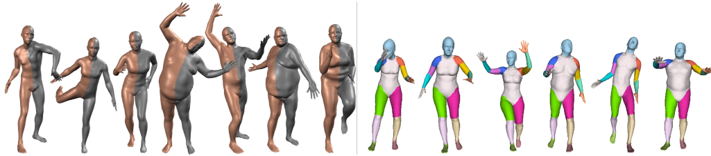
Figure 2.4: On the left, some examples of the body poses and shapes using SMPL body model. The image shows the body pose estimated using SMPL model configuration (brown) vs the ground truth 3D scan model (gray). On the right, some examples of the poses and shapes using Stitch body mode. Each colour represents a different deformable body part.
