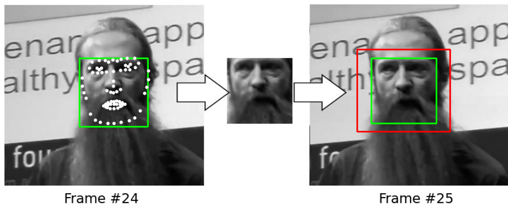
Figure 4.7: Representation of the face location update between the frames #24 and #25 of the sequence 410 of the '300VW challenge' dataset [127]. The tracker extracts the face template (middle) from the frame #24 using the projection of the 3D vertices. Then, it finds the template in the red area in the frame #25.
