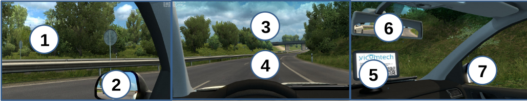
Figure 6.5: The considered zones of interest in the simulator to analyse the driver's PoG.
