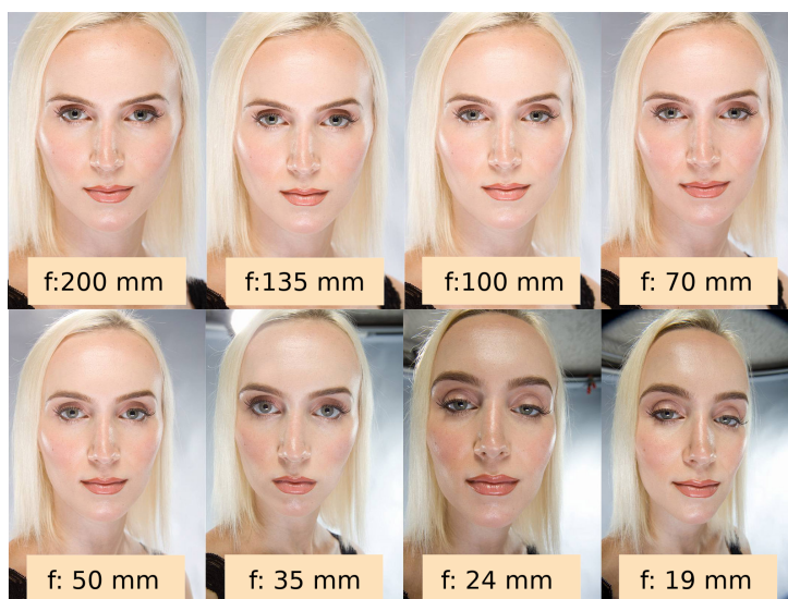
Figure 2.17: Different images of the same face taken with a full-frame camera and using objectives with different focal lengths. Original image by Stephen Eastwood 3
