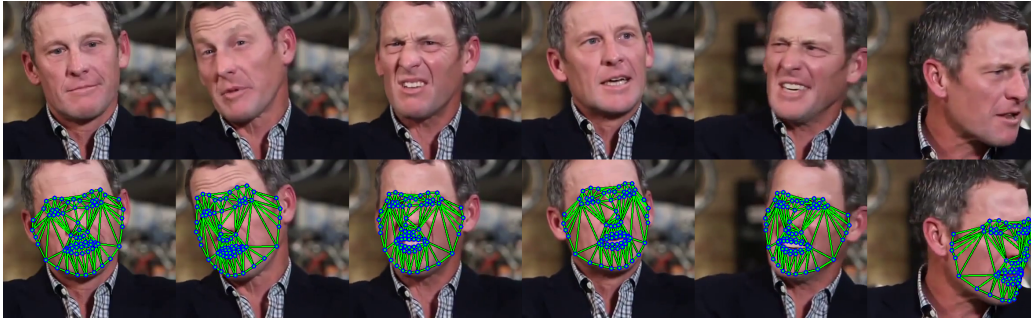
Figure 1.3: A tracked sequence (from left to right) of a face using an automatic 3D face tracker. The upper row shows the original image captured by a colour camera and the lower row shows the same images with a 3D face model overlapping the face representing the tracking output.
