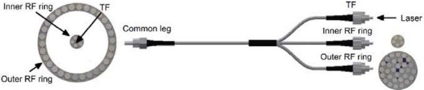
Figure 20: Photograph of each of the ends and schematic of the of the upgraded manufactured fiber bundle.
