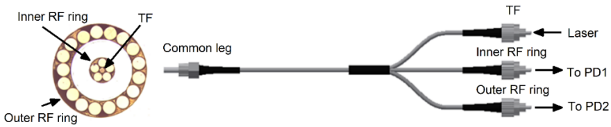
Figure 14: Photograph of the end face of the probe tip and schematic of the manufactured fiber bundle.
