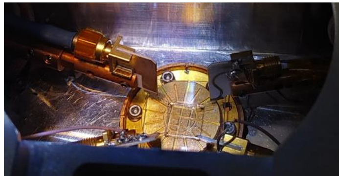
Figure 2.10 Photo of the Van der Pauw measurement setup.
