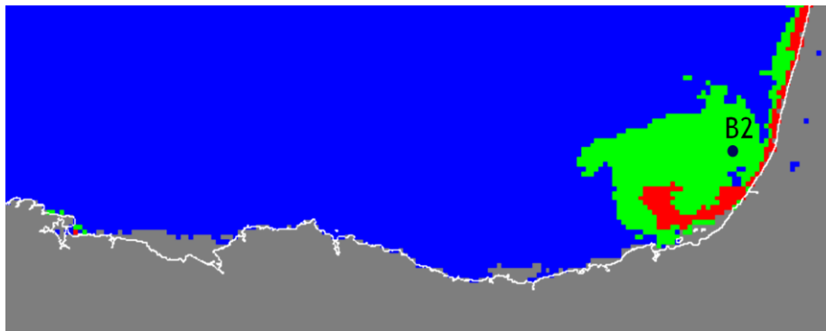
Figure 3.11. K-means cluster classification of the Basque coastal water bodies using reflectance bands of the MERIS FR products acquired on the 5 th of June 2007. Class I corresponds to the red colour, class II to the green colour and class III to the blue colour. Station B2 was sampled on that date and included in the classification analysis of the biogeochemical and optical data.
