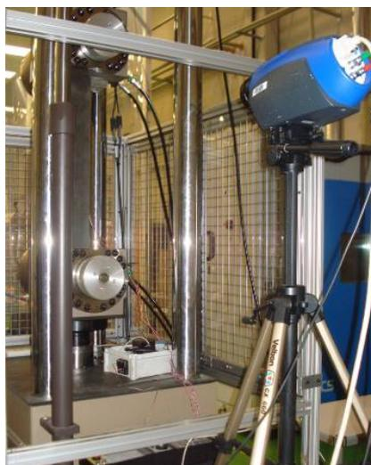
The specimen has been subjected to different types of stress fatigue, varying the frequency of cycling and stress limits:
