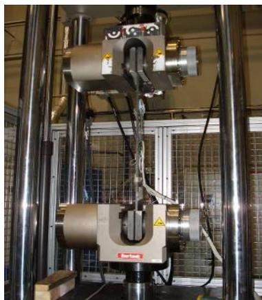
This machine applies the scheduled stresses or strains through four hydraulic actuators at a maximum force of 500 kN. Load levels chosen for the tests were such that there is no risk of causing plastic deformations on specimens and test safety was not compromised.
