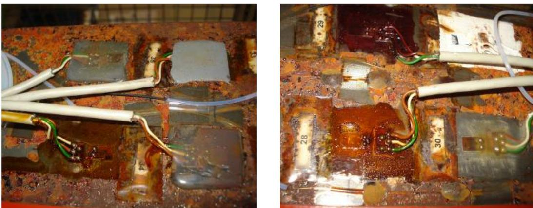
The second series of tests consisted of traction and compression tests on the three specimens with the loading levels discussed above. When performing the pretest with specimen 1, there was a breakage after FBGs number 6, with the consequent invisibility of FBG sensors 7, 8, 9 and 10.
