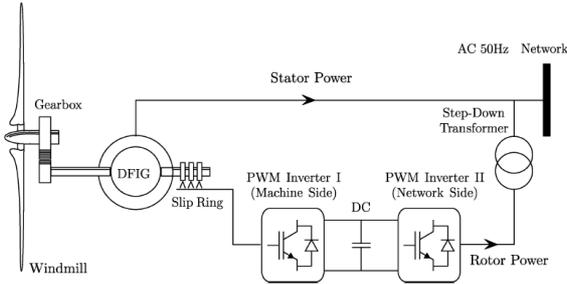
**Figure 2. Scheme of a DFIG equipped wind turbine**
