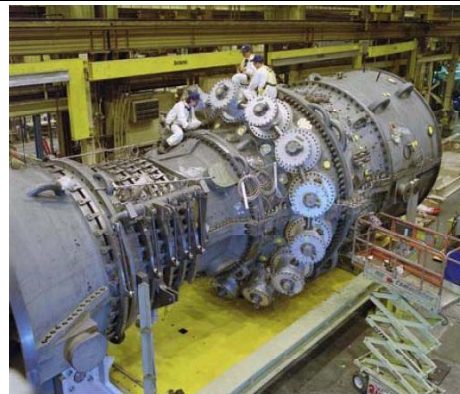
GE-9H gas turbine is prepared for testing (Source: GE Power Systems)
