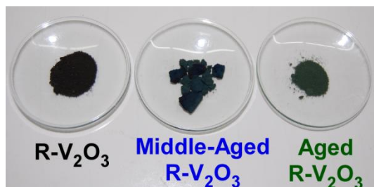
Figure 2.34 External aspect of R- \text{V}_2\text{O}_3 , Middle-Aged R- \text{V}_2\text{O}_3 and Aged R- \text{V}_2\text{O}_3 vanadium (III) oxides.
