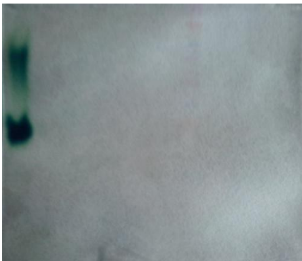
Figure 13: The zymography made in a 15% polyacrilamide gel. The positive control took a green color which shows the laccase activity. The protein samples obtained from gave no signal.
