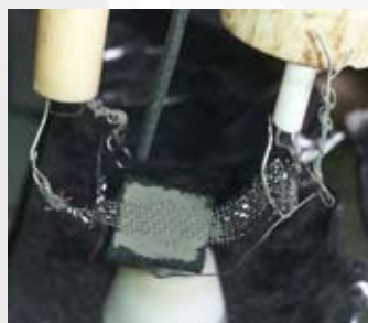
Figure 1. Interconnect/contact layer/cathode system.
