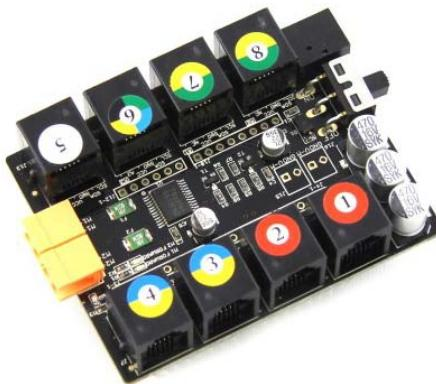
You can easily connect Me Series Electronic Modules to Arduino board through the Base Shield. With a TB6612 motor driver IC on board, it can drive 2 DC motors.
