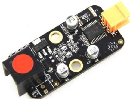
Me-Motor Driver could drive a DC motor with a RJ25 port which contains power lines and signal lines. The wiring has been simplified.
