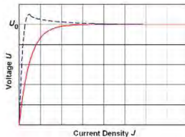
Figure 4-35 Voltage-Current density principle for an electrical conductivity in the splitter plate shell [53]
