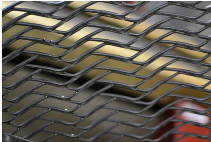
Fig. 2.13. EM mesh obtained when: blade's horizontal movement < LW/2 .
