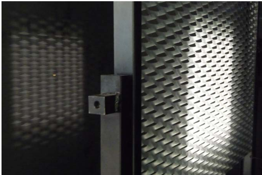
Fig. 5.14. Projected shadow pattern projected through a mesh (without diffuser layer)
