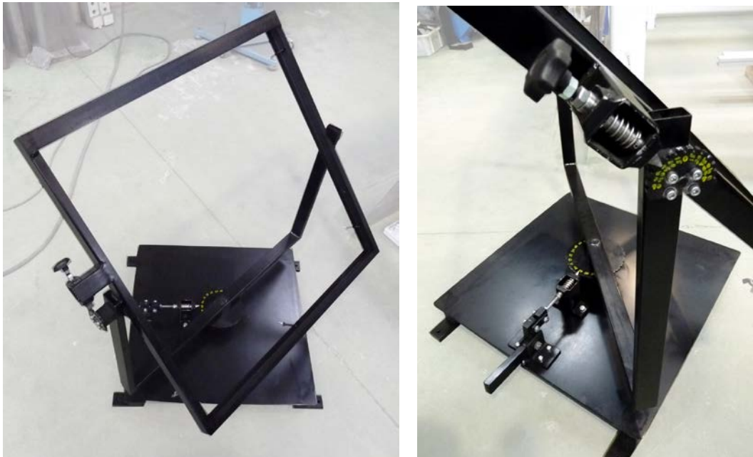
Fig. 5.10. Left: Rotary sample holder. Right: Sample holder's rotation and fixing systems
