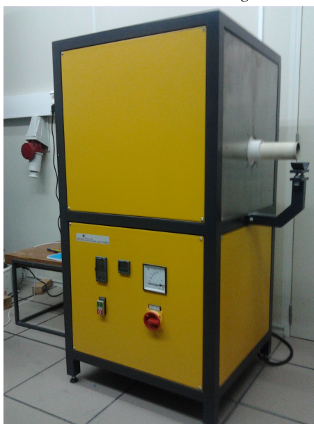
Figure B.2: AGNI Ceram-Aix RHT 175-50-300-1H furnace ( UPV/EHU: Applied Physics II department )
