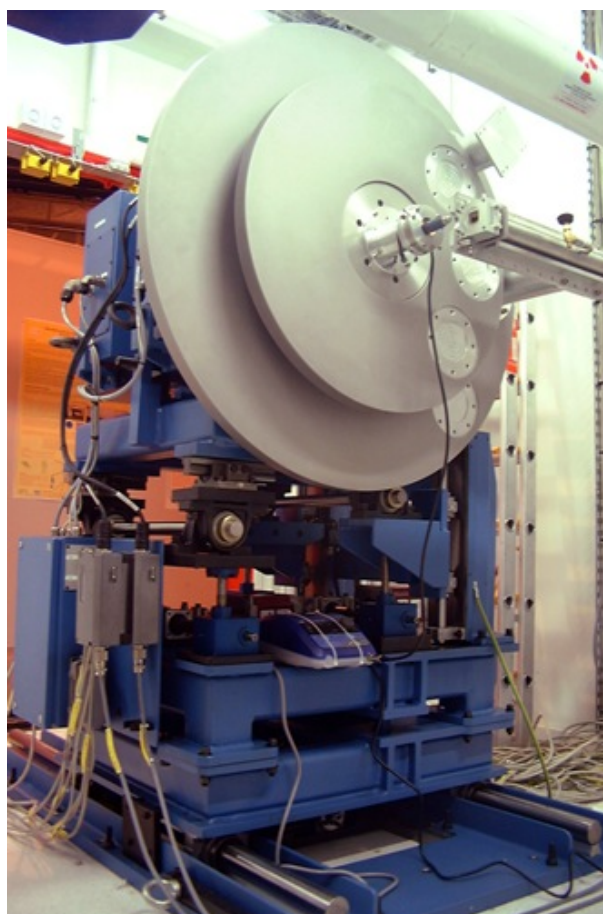
Figure B.9: Powder diffractometer from BM25-Branch A line in ESRF.
