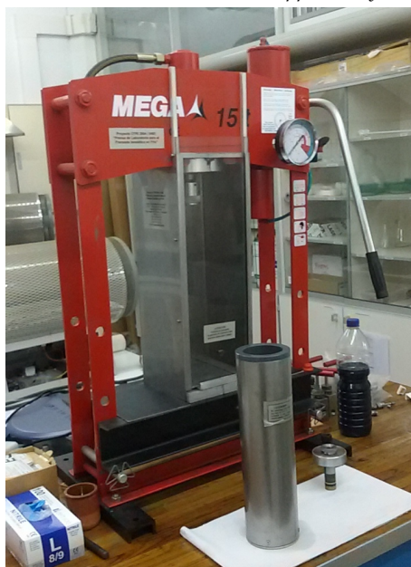
Figure B.4: MEGA KSC-15 press, with a capacity of 15t (UPV/EHU: Inorganic Chemistry department)
