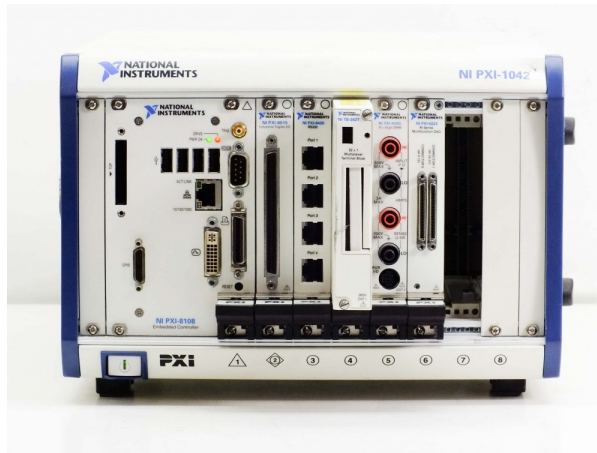
Figure 3.1. – A 18 slot PXI chassis, with a controller in the left side of the picture and 8 modules installed.
