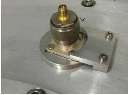
Figure 5.16. – One of the two coupled pickups of the resonant cavity.
