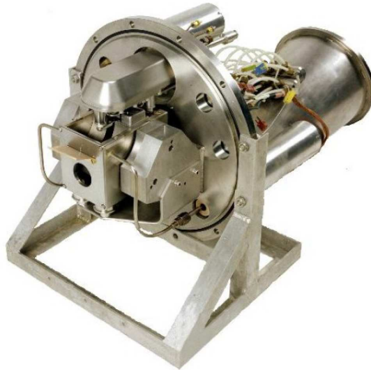
Figure 1.2. – A Penning ion source of the the Front End Test Stand (FETS) experiment at the Rutherford Lab.
