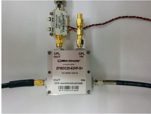
Figure 5.12. – Bidirectional coupler and power detector at the coupled reverse port to measure the reflected signal voltage
