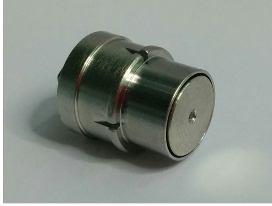
Figure 4.6. – Picture of the used capacitive pick-up sensors. The metallic plate can be observed.
