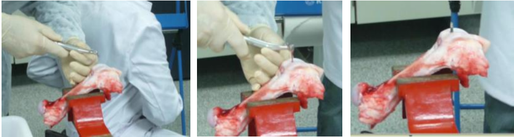
Figure 8.1. Resistance test to the surgically implantation process in pig knee bone.
