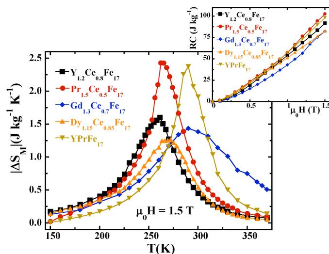
Figure 3. Temperature dependence of the magnetic entropy change for  $\text{R}_x\text{R}'_{2-x}\text{Fe}_{17}$  alloys under  $\mu_0\Delta H = 1.5$  T. Inset shows the field dependence of refrigerant capacity.
