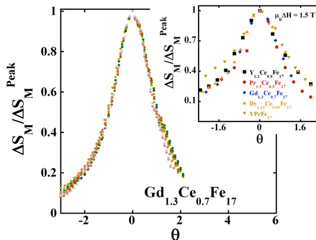
Figure 4. Master curve for  $\text{Gd}_{1.3}\text{Ce}_{0.7}\text{Fe}_{17}$  obtained using two temperatures of reference (see text for details). The inset shows a comparison of the master curves for the studied pseudo-binary alloys under a magnetic field change  $\mu_0\Delta H = 1.5$  T.
