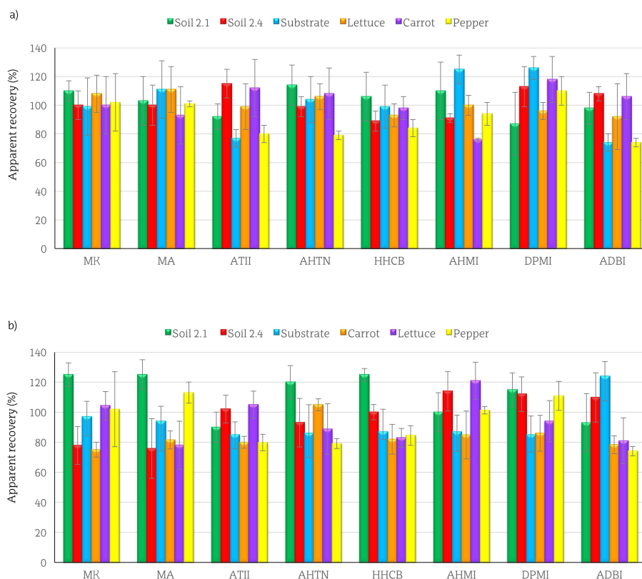
Figure 4.6. Average recoveries (%) and their deviation using matrix-matched calibration and ^2\text{H}_{15} -MX as surrogate for a) low ( n=7 , 95 % confidence level) and b) high ( n=4 , 95 % confidence level) concentration levels.
