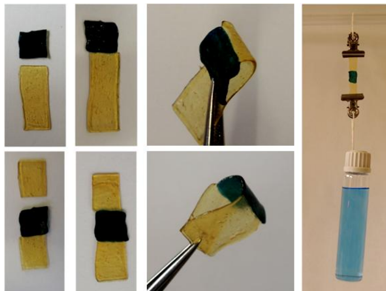
Figure 5.4 Qualitative analysis of the healing abilities of PPGDHMC samples. Methylene blue was used for visibility.
