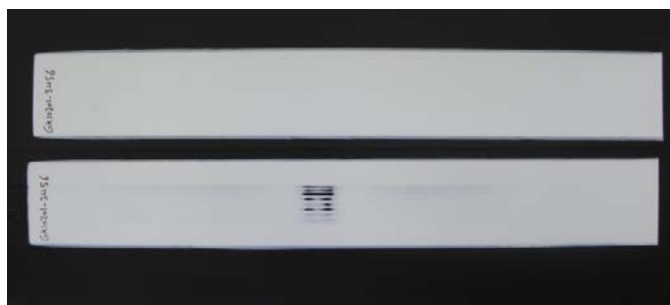
Fig. 5.10. Picture of the paint films from Run 3D latex before (up) and after (down) the scrub test.
