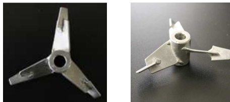
Figure 2. 6. Ekato Mig impeller bottom (left picture) and side (right picture) view.
