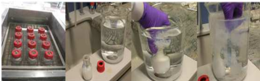
Figure 2. 4. Sequence of steps for removing the non deposited latex after the experiment.
