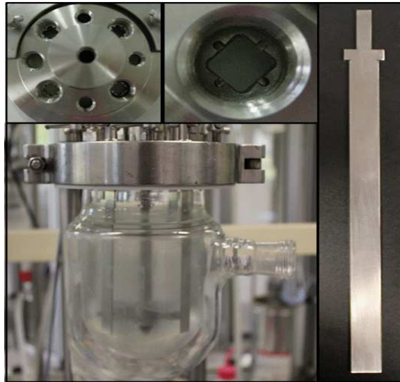
Figure 4. 1. Reactor used to study orthokinetic fouling.
