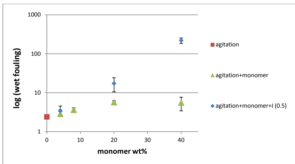
Figure 5. 4. Comparison of the wet fouling measured after polymerization (agitation+monomer+I 0.5 wt%) with that observed without reaction (agitation+monomer).
