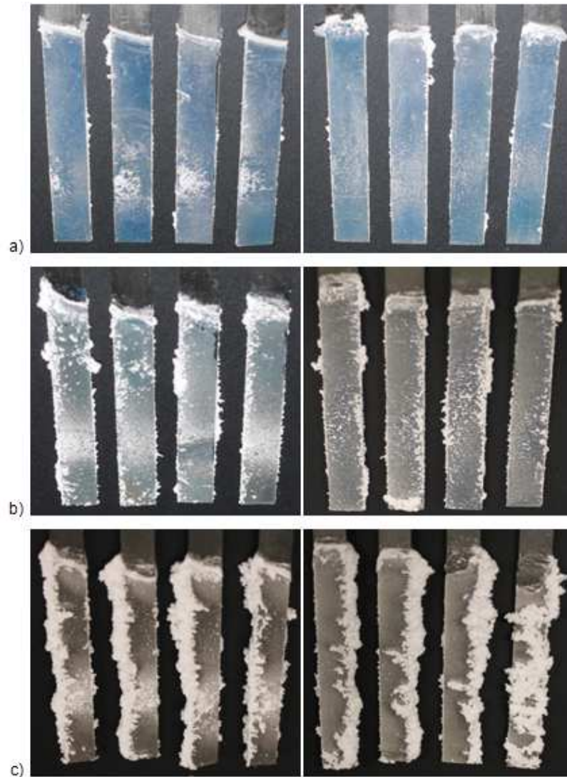
Figure 5. 5. Fouled substrates for the 96/4, 80/20 and 60/40 ratios under reaction by the addition of 0.5 wt% monomer based KPS.
