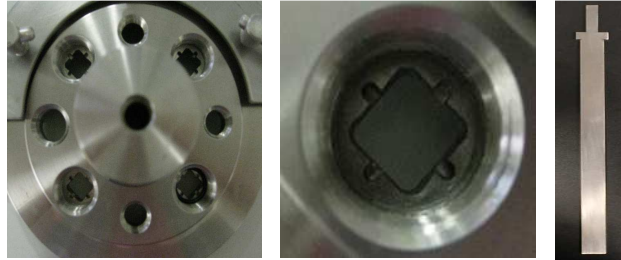
Figure 2. 5. Reactor lid designed, zoom of a substrate holder and stainless steel substrate.
