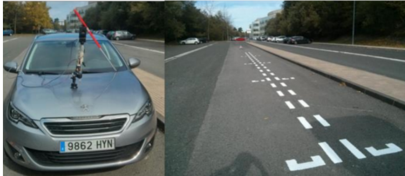
Figure 24: Physical car setup
