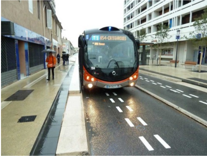
Figure 3: eBRT riding with lane marking system
