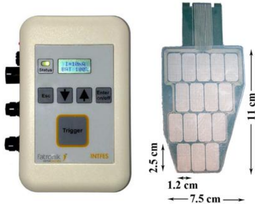
Figure 4.1: IntFES stimulator [58] and multi-field electrode[59] .
