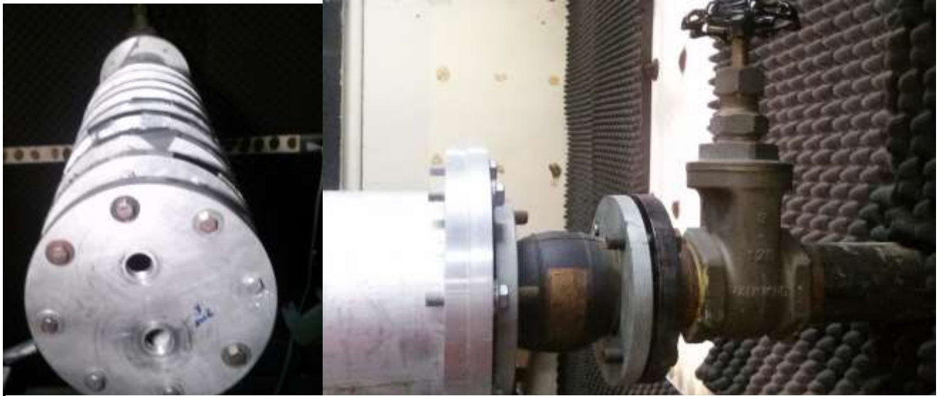
Figure 11: Compressed air jet and control valve
