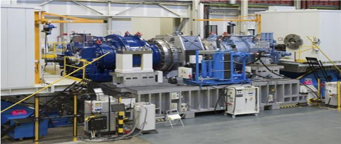
Figure 2.14: Back to back test rig
