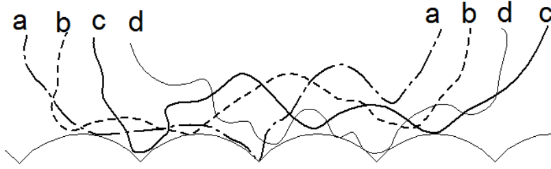
Figure 2.7: Surface created by the dresser on consecutive grains [CR96]
