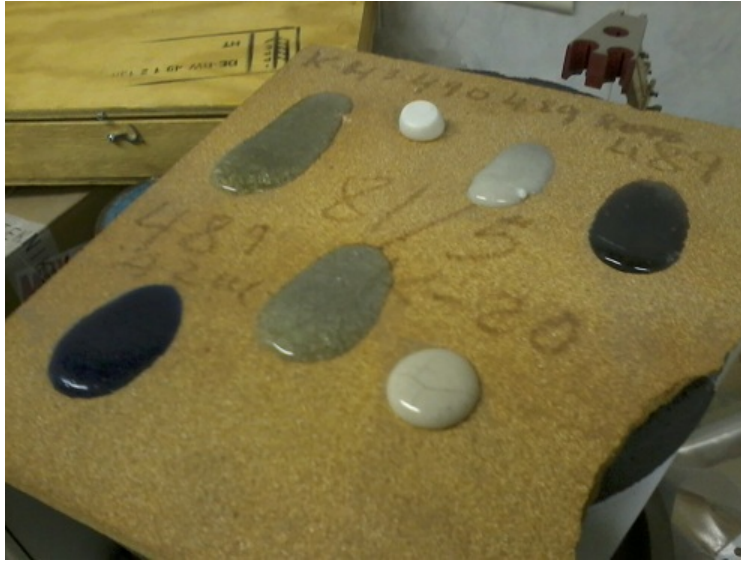
Figure 3.11: Drop test of the binder: the viscosity is verified measuring the spread distance in a given slope (source: Unesa)
